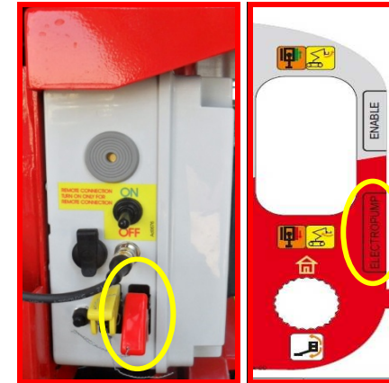
Picture 29: electropump activation buttons.
