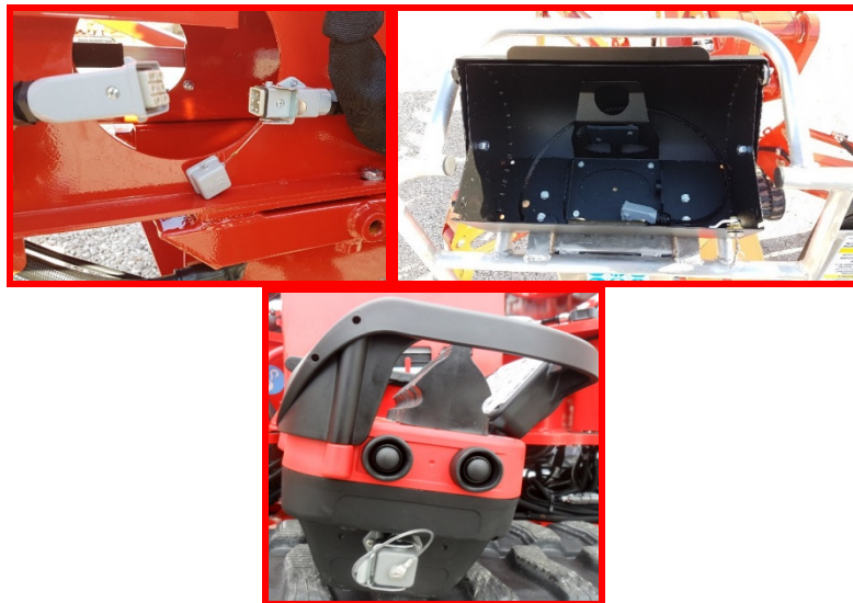
Picture 11: frame and basket connectors for wired remote control.
